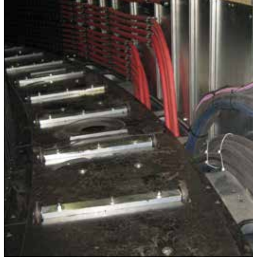
Rotary system with “floating islands” for safe operation on rough seas – rotation angle 540°
