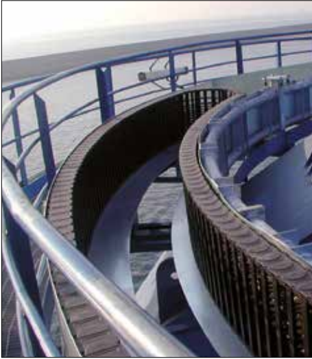
Opposing series 5050 e-chains® with igus® guide trough system and support structure – outer diameter: 39.4 ft., rotation angle: 340°.
